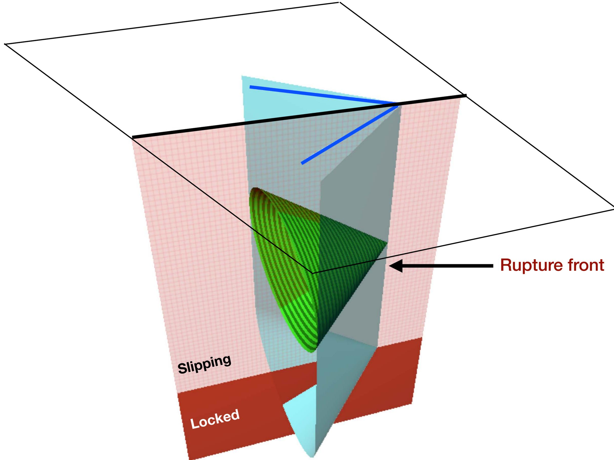
Shear Mach cone from a generic point on the rupture front
